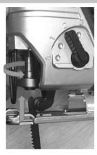
Important! : Make sure the saw blade sits properly in the slot of the roller and groove.
